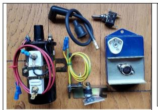
Mount the coil & ECM within reach of their various connections. 12V via toggle switch is applied to the  $\frac{1}{2}$  female QC at back of coil.
