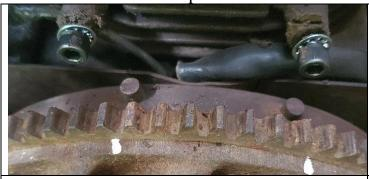
Install (2) 1/4-20 socket head fasteners & star washers Mark Long (TDC) & Short (ADV) pins for later use
