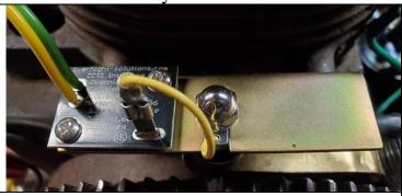
Mount CCTI Interface/Magnetic pickup & set the gap between the Magnetic Pickup & Long pin to 0.010"
