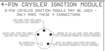
Female bullet QC connections made to ECM as defined above. Make certain that the leads will reach before mounting components. Toggle switch can be mounted anywhere as wires are cut to length.
